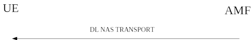
Figure 5.4.5.3.2.1: Network-initiated NAS transport procedure
