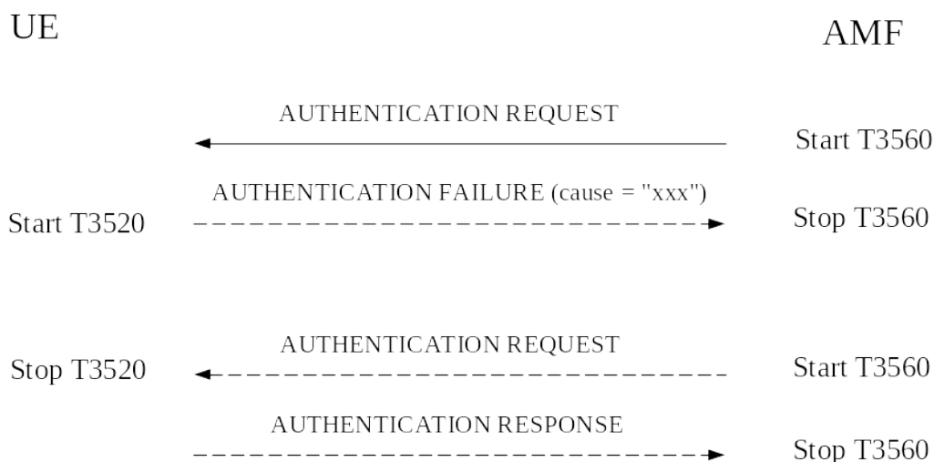
Figure 5.4.1.3.7.1: Authentication failure during 5G AKA based primary authentication and key agreement procedure
