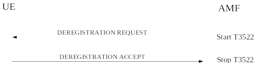
Figure 5.5.2.3.1.1: Network-initiated de-registration procedure
